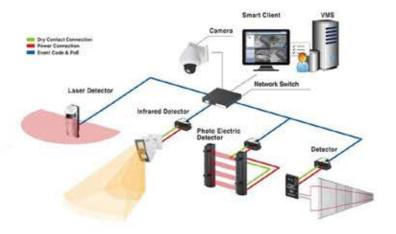
A passive Infrared Sensor (PIR sensor) is an electronic sensor that measures infrared (IR) light radiating from objects in its field of view.
